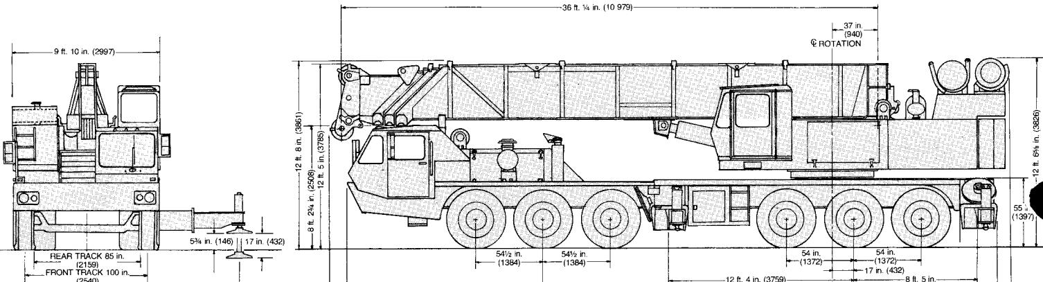
Main hoist with 750 ft. (228.6 m) of ¾ in. (19 mm) rope, 12 x 6 – 100 carrier, Cummins NTC 350 (carrier engine), Cummins V555-C230 (superstructure engine)
