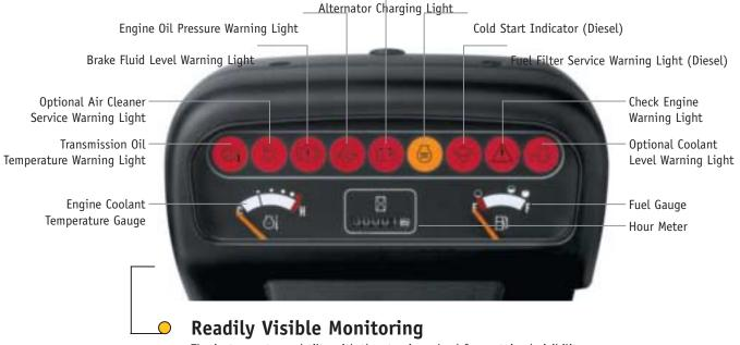
The instrument panel tilts with the steering wheel for sustained visibility and provides easy monitoring of truck functions plus early warnings of potential problems to promote preventive maintenance.
